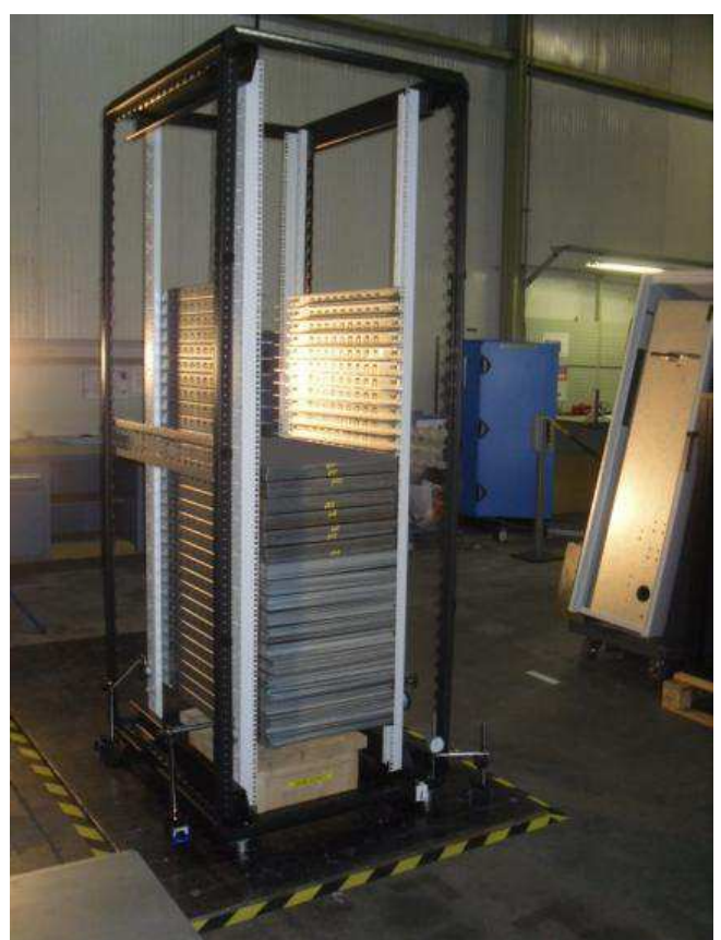
Picture 2 Frame loaded with 2000 kg
