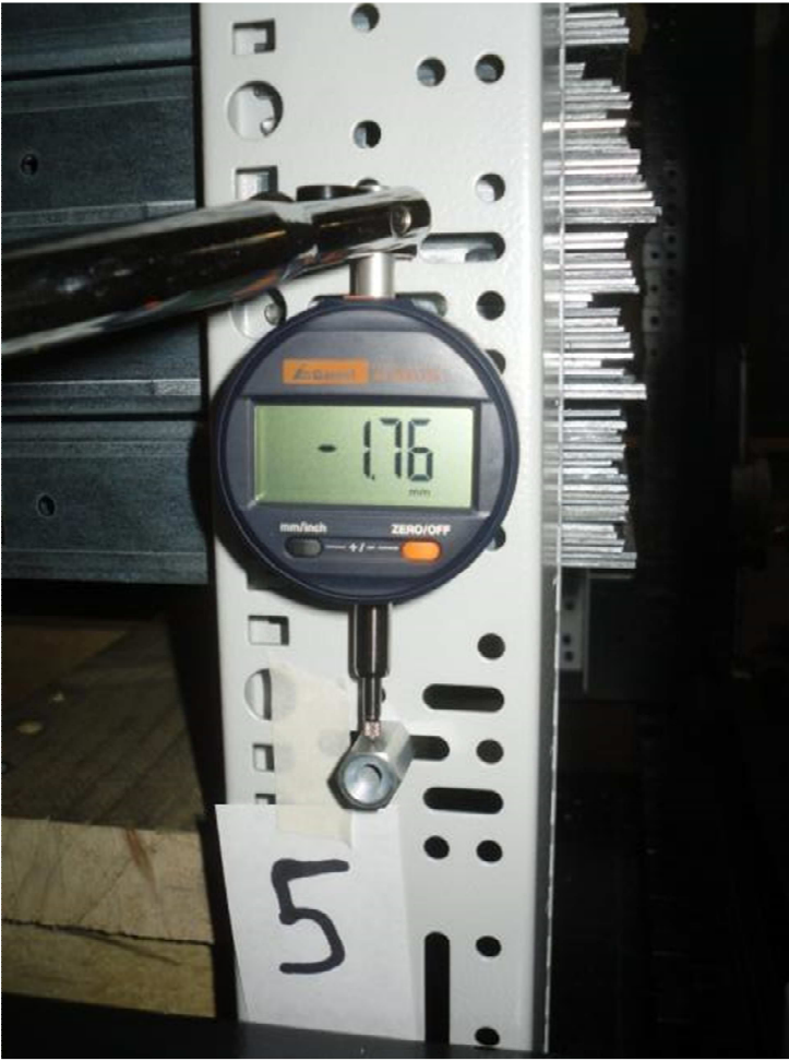
Picture 3 Dial indicator to measure panel mount displacement
